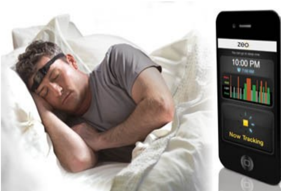
Sleep subjects will use a wireless brain monitor with three sensors incorporated into a headband that will interface with a smartphone.
